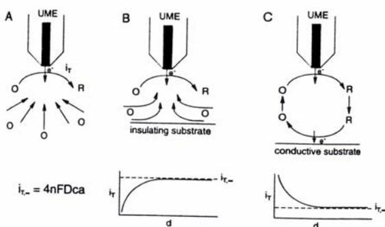
**Figure 1.** Operating principles of SECM. (A). With UME far from the substrate, diffusion of  $O$  leads to a steady-state current,  $i_{T,\infty}$ ; (B). With the UME placed near an insulating substrate, hindered diffusion of  $O$  leads to  $i_T < i_{T,\infty}$ ; (C). with UME near a conductive substrate, positive feedback of  $O$  leads to  $i_T > i_{T,\infty}$ . Graphs: current,  $i_T$ , as a function of tip location. A particular advantage of SECM in imaging
