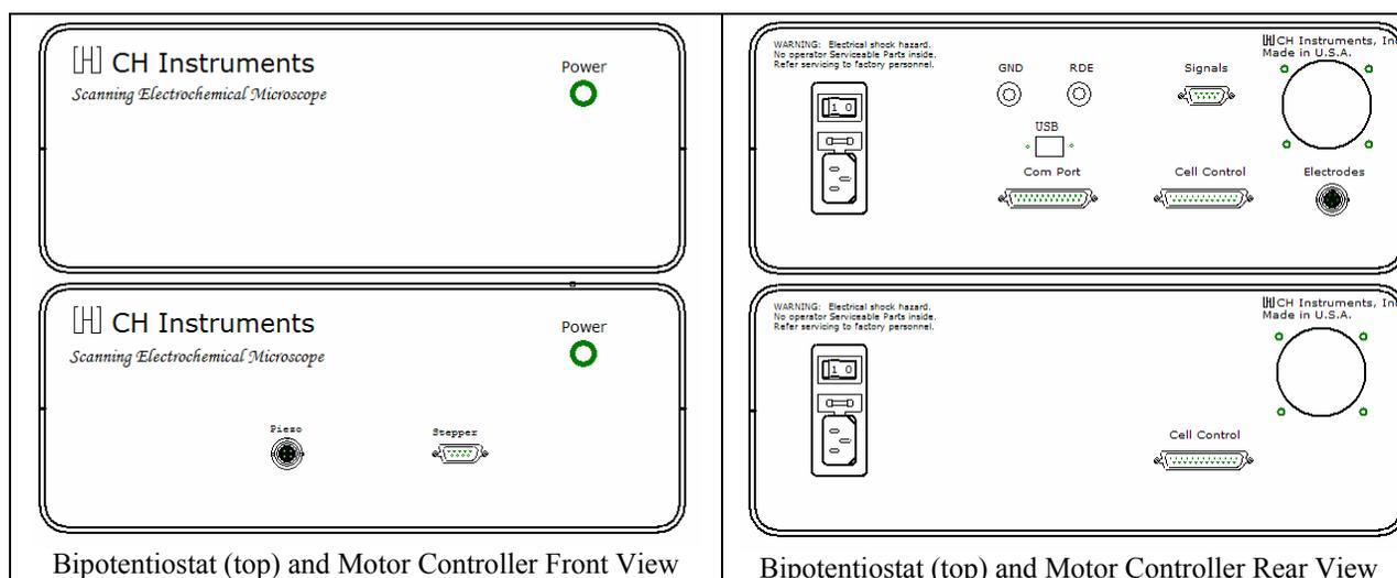
Bipotentiostat (top) and Motor Controller Front View
