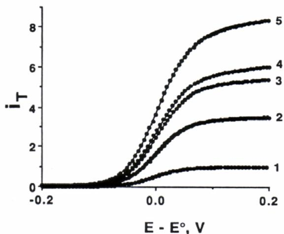
**Figure 3.** Tip steady-state voltammograms for the oxidation of 5.8 mM ferrocene in 0.52 M  $\text{TBABF}_4$  in MeCN at a 1.1- $\mu\text{m}$ -radius Pt tip. Solid lines are theoretical curves and solid circles are experimental data. Tip-substrate separation decreases from 1 to 5 ( $d/a = \infty, 0.27, 0.17, 0.14, \text{ and } 0.1$ ). (Reprinted with permission from Ref. 4e, copyright 1993, American Chemical Society.)
