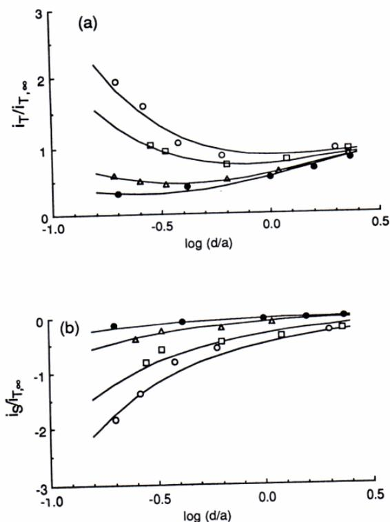
**Figure 5.** Normalized tip (generation, A) and substrate (collection, B) current-distance behavior for FN reduction. FN concentration: (open circle) 1.50 mM, (open square) 4.12 mM, (open triangle) 28.2 mM, and (filled circle) 121 mM.  $a = 5 \mu\text{m}$ , substrate radius is  $50 \mu\text{m}$ . The solid lines represent the best theoretical fit for each set of data. (Reprinted with permission from Ref. 5a, copyright 1992, American Chemical Society.)
