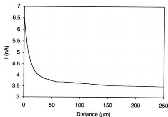
**Figure 8.** Approach curve for the system: 10 mM TCNQ and 1 mM  $\text{TPAsTPB}$  in DCE // 1 mM  $\text{Fe}(\text{CN})_6^{3-}$ , 0.1 M LiCl and 1 mM  $\text{TPAsCl}$  in  $\text{H}_2\text{O}$ , showing reverse electron transfer driven by phase transfer catalyst  $\text{TPAs}^+$ . Tip potential, -0.4 V vs Ag/AgCl. (Reprinted with permission from Ref. 7c, copyright 1995, American Chemical Society.)
